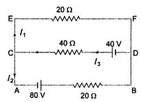
14. In the circuit shown in the figure, find the total resistance of the circuit and the current in the arm CD.
